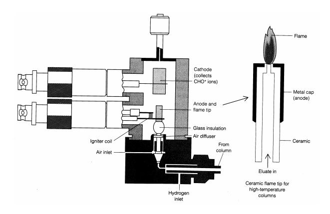
In the flame ionization detector, eluate is burned in a mixture of  $H_2$  and air:
