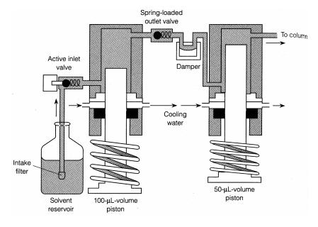
Typically HPLC instruments have two pumps which work in tandem. If a gradient mobile phase is employed in order to produce the correct ratio of the mobile phase solvents.
