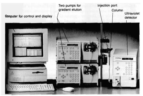
**HPLC** uses high pressure to force eluent through a closed column packed with micron-size particles.
