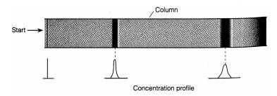
A band of solute invariably spreads as it travels through the column and emerges at the detector with a standard deviation,  $\sigma$ .
