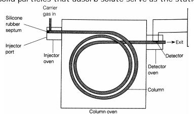
A volatile liquid is injected through a rubber **septum** into a heated port which vaporizes the sample. The sample is swept through the column by He, N<sub>2</sub> or H<sub>2</sub> *carrier gas*, and the separated solutes flow through a detector.
