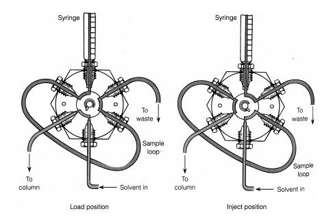
The sample injector portion shown for the HPLC is a closed system. By rotating the injector lever, the analyte is introduced to the mobile phase. The mobile phase carries the analyte on to the HPLC column where the separation begins.
